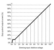
$\bigcirc$  Applying additive 10V PWM signal (frequency range 300~3KHz):
