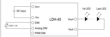
During analog dimming operation, Io will change with DC input voltage
